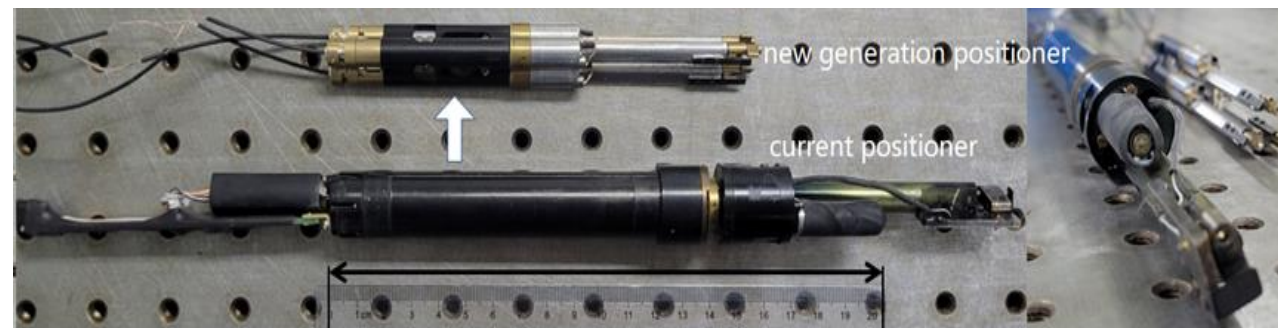
Comparison with two generations of fiber positioners
